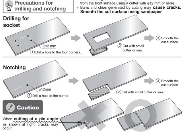
•In the case as shown at upper right, select allocation with multiple pieces instead of notching.
